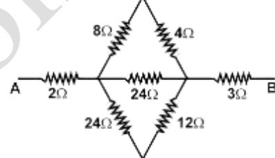
Q10. Find the effective resistance of the given circuit between A and B. [Ans.  $\frac{97}{5}\Omega$ ]
